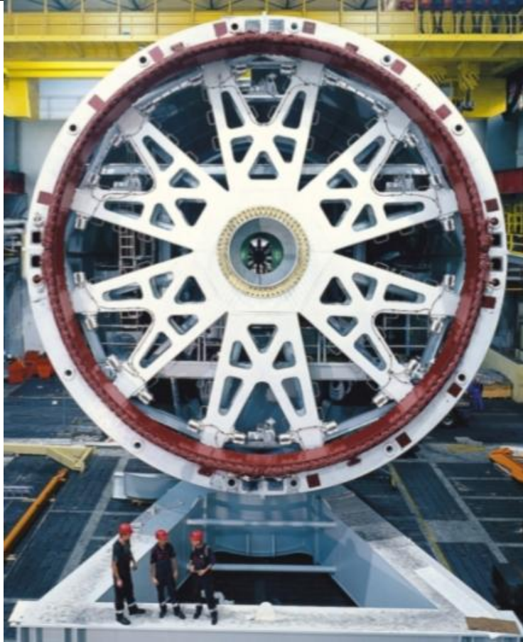
Enercon E-126 – 7.58 MW Direct Drive Wind Turbine Annular Generator
